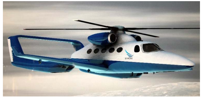
Skyworks announced its VertiJet tipjet-powered civil gyroplane on Feb. 1. It leverages the Groen Brothers technology from the DARPA Heliplane program. (Skyworks image)
