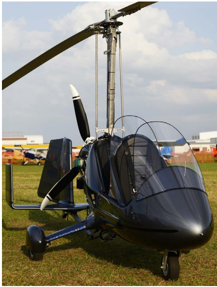
Silverlight Aviation's American Ranger 1 (AR1) gyroplane has with tandem seating and is convertible from fully enclosed or open windshields. (Silverlight photo)
