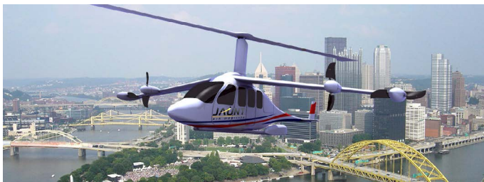
The Jaunt Air Mobility air taxi leverages the technology developed by Carter Aviation Technologies for its slow rotor/compound gyroplane. Jaunt is developing an all-electric VTOL air taxi for the Uber Elevate mission. (Jaunt image)
