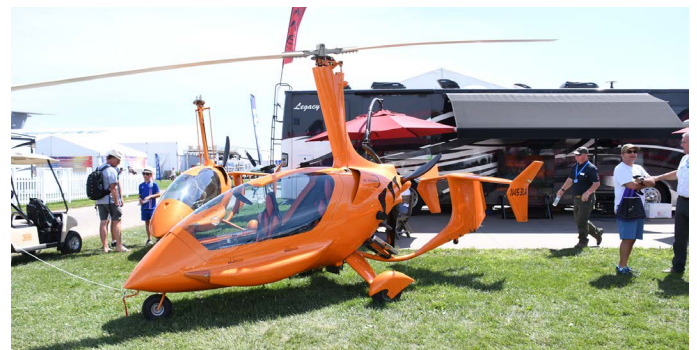
The ELA Aviación ELA 10 Eclipse is a two-place gyroplane introduced at the in 2014. (VFS photo by Ken Swartz. See more gyroplane photos from EAA AirVenture 2018 in the Vertical Flight Gallery at www.gallery.vtol.org .)
