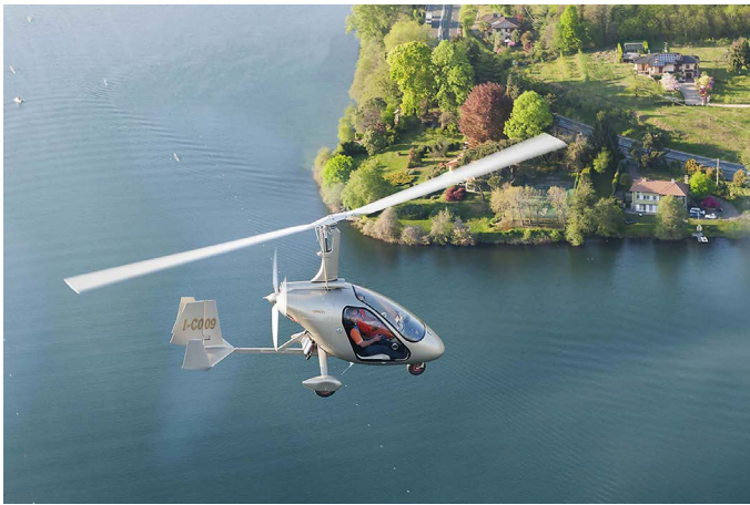
The Magni Gyro M24 Orion is an enclosed side-by-side gyroplane. (Magni photo)
